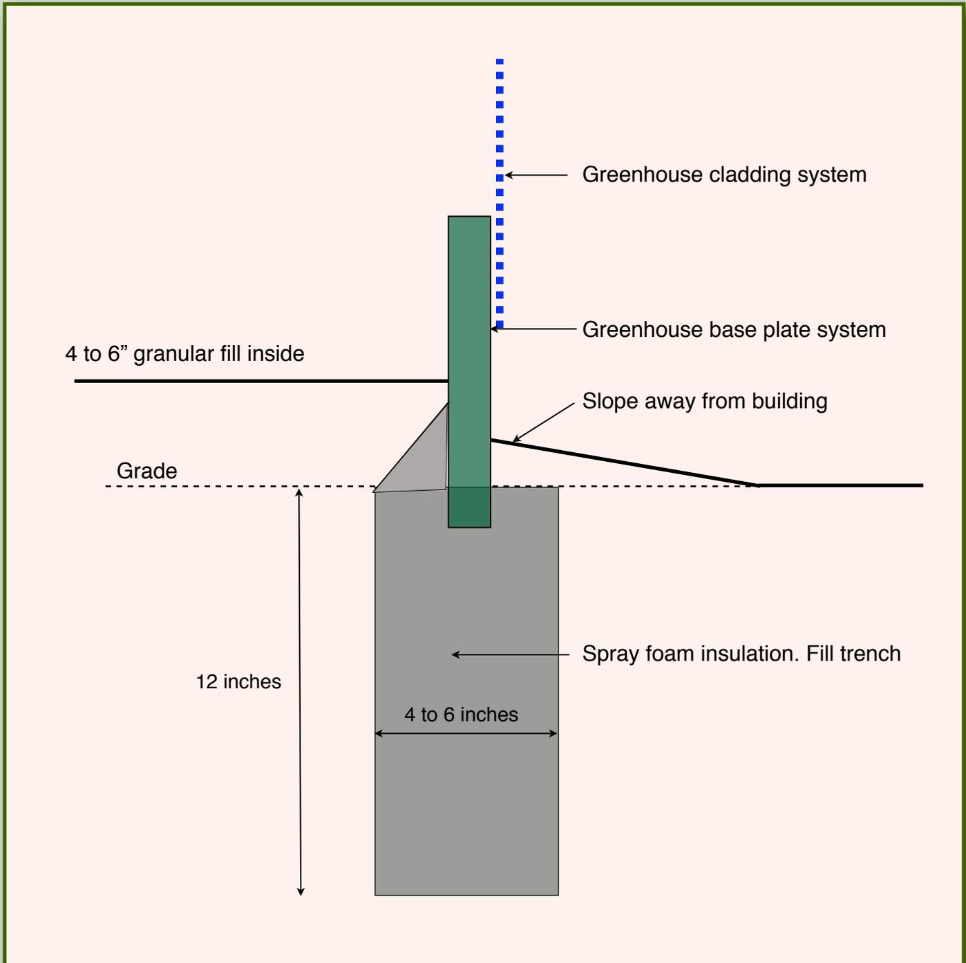
**Concept Sketch.** Cut trench method for soil thermal break and base infiltration protection. For detailed construction plans/details contact our office. File no. 801011. Cad/pdf format available.
