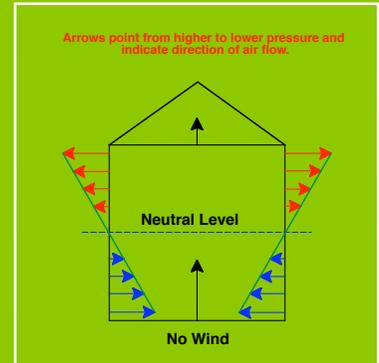
Is the uncontrolled flow of air through openings in the building envelope driven by pressure differences across the shell. Infiltration is balanced by an equal amount of exfiltration. Uncontrolled/excessive infiltration will contribute greatly to your heating costs.
