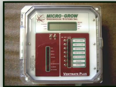
heating for a single zone. Don't let the size fool you. There is a lot of power at your finger tips. It will provide cooling and dehumidification control, heating control, control of your HAF fans, provide DIF control if desired and allow you to program in four temperatures and humidity set points for various times of the day, which are programmable.
